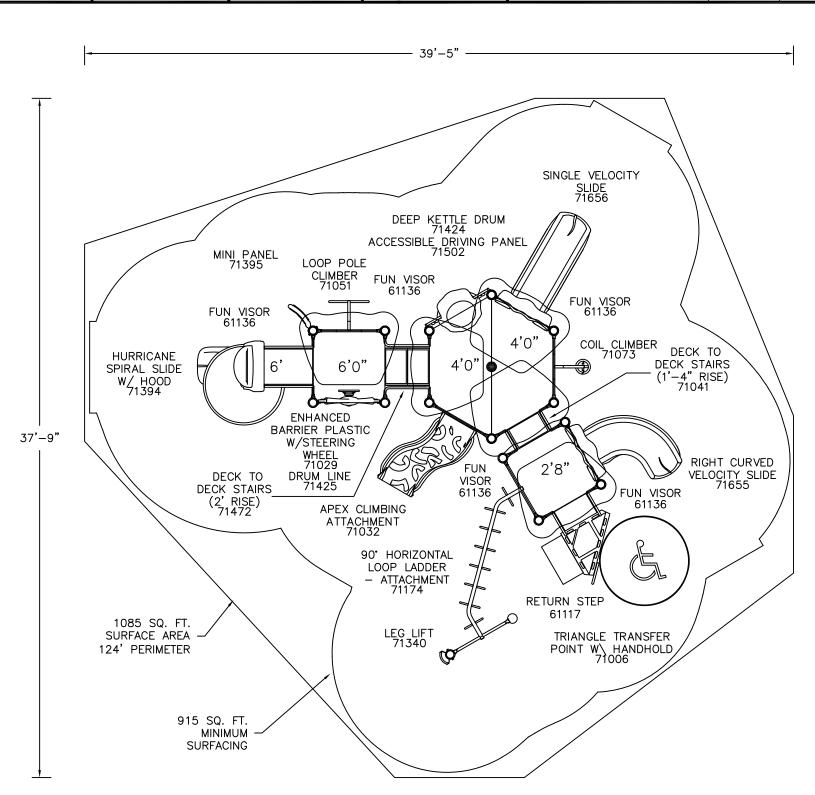
It is the manufacturer's opinion that the structure shown herein complies with current ada standards concerning accessibility if used with proper accessible surfacing and together with other necessary ground level play equipment.
